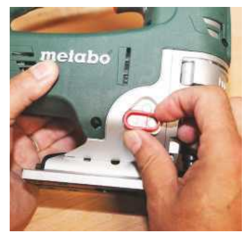
▲ The blower switch is similarly cheap looking and is a simple on-off function
